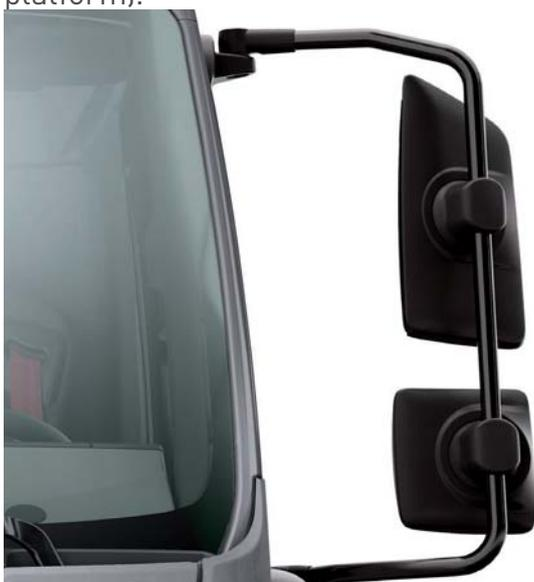
**DE-ICING AND ELECTRICALLY ADJUSTED REAR-VIEW MIRRORS**
